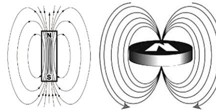
The detection range depends on the strength of the magnet, so its physical size. It is also important to consider the magnet placement to obtain the strongest magnetic field. For short distance, use a smaller magnet to avoid sensor overdrive.
