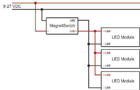
The diagram above is an example of the connection and may be different from the actual layout. Wires between the power supply, controller and LED modules should be as short as possible. Connecting more than one controller to the same power supply is not recommended. It may cause interference, visible on LED light sources. Controllers adapted to such work are available on special request.
